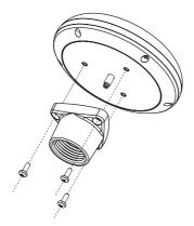
Figure 2.3.0 - Installing the External GPS Antenna (I)
